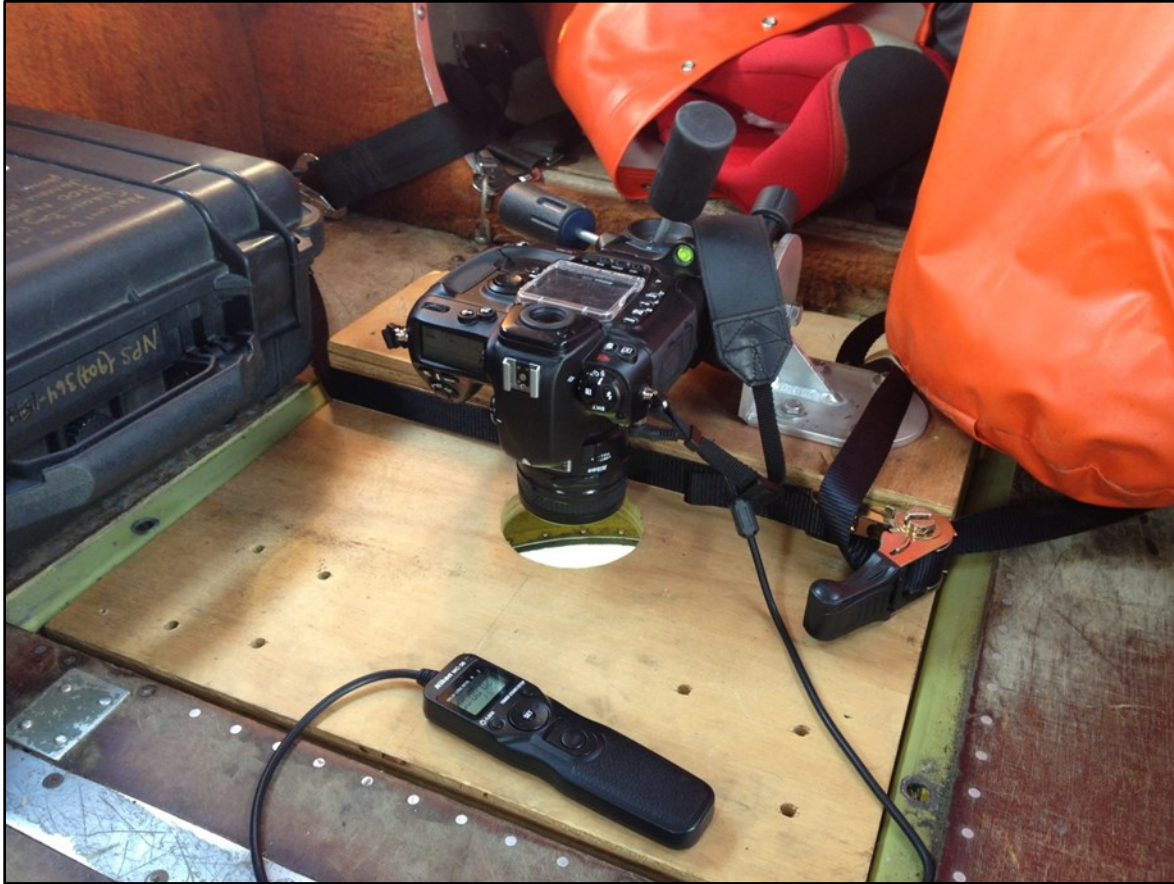
Figure 3.2. Digital camera mounted on tripod head and attached to custom-made plywood frame and secured in the belly of the aircraft. Plywood frame is secured to plane using cargo straps.
